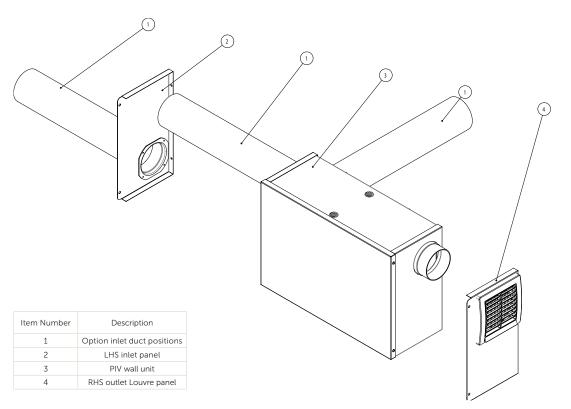
Inlet options from left hand side. Outlet Louvre accessory shown right hand side.
